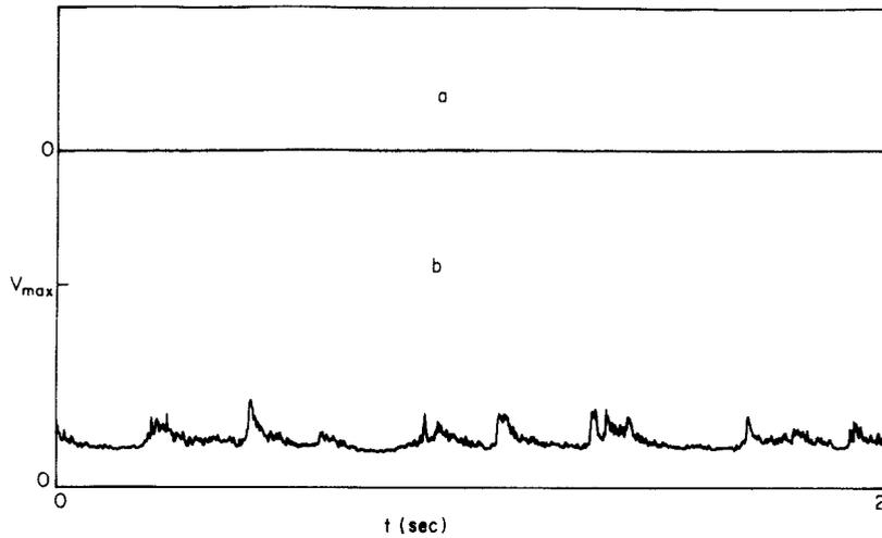
Figure 6. Annular flow,  $u_{Gs} = 30$  m/sec,  $u_{Ls} = 0.048$  m/sec, horizontal.
