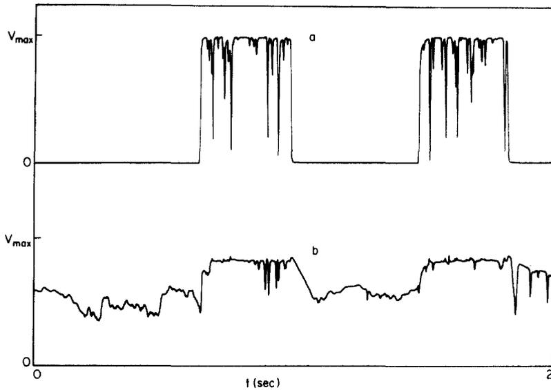
Figure 10. Slug flow,  $u_{G,s} = 0.3$  m/sec,  $u_{l,s} = 0.03$  m/sec, vertical upflow.
