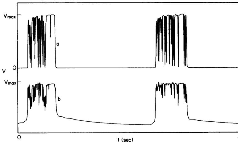
Figure 3. Slug flow,  $u_{Gs} = 1.2$  m/sec,  $u_{Ls} = 0.48$  m/sec, horizontal.
