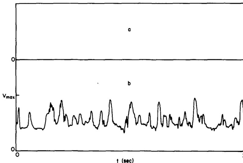
Figure 13. Annular flow,  $u_{Gs} = 12$  m/sec,  $u_{Ls} = 0.03$  m/sec, vertical upflow.
