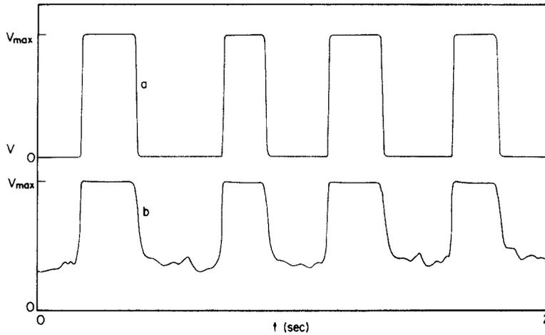
Figure 2. Elongated bubble flow,  $u_{Gs} = 0.12$  m/sec,  $u_{Ls} = 0.48$  m/sec, horizontal.
