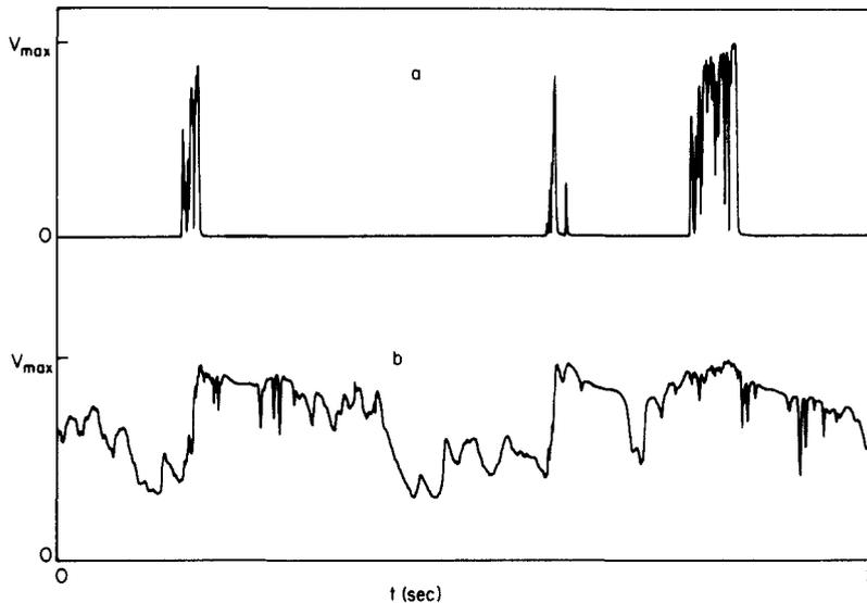
Figure 11. Churn flow,  $u_{G,s} = 1.9$  m/sec,  $u_{l,s} = 0.03$  m/sec, vertical upflow.
