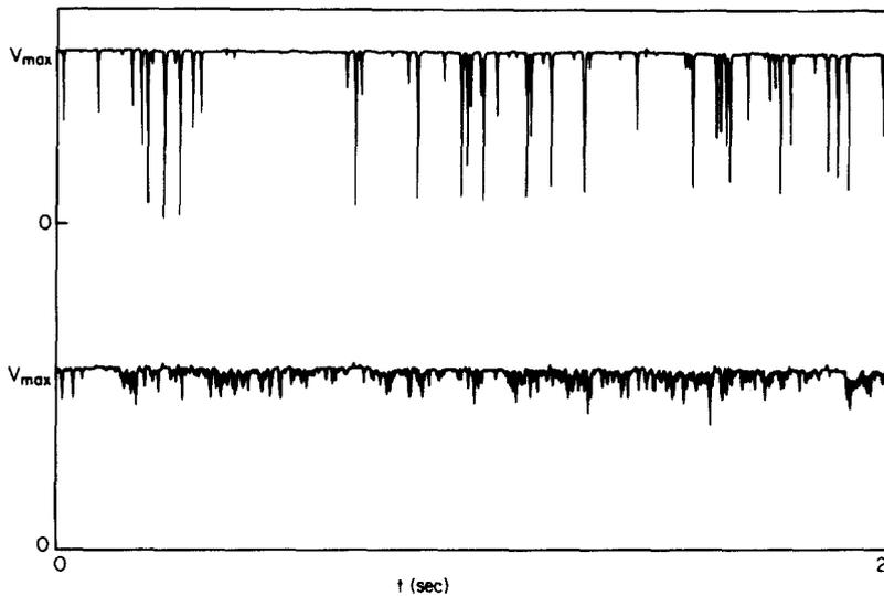
Figure 14. Dispersed bubble flow,  $u_{Gs} = 0.3$  m/sec,  $u_{Ls} = 1.9$  m/sec, vertical upflow.
