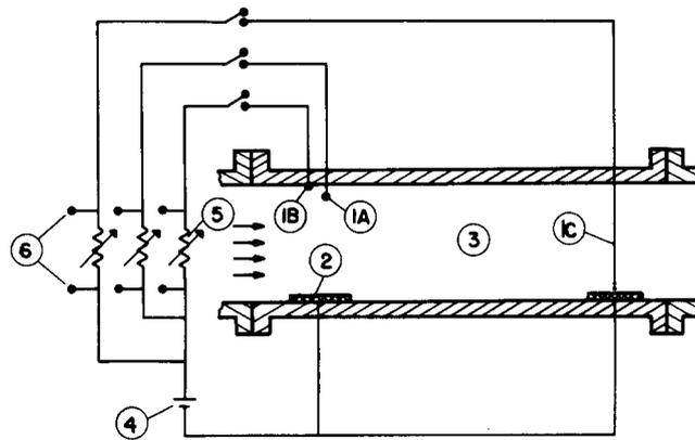
Figure 1. Scheme of probing system. (1A) Probe—Tip electrode, stainless steel wire, 0.25 mm dia., teflon coated, 3 mm down from tube top; (1B) Probe—Tip electrode, stainless steel wire, 0.25 mm dia., teflon coated, flat with tube surface; (1C) Probe—Metal needle, not insulated; (2) Flat copper electrode; (3) Two-phase flow; (4) Voltage supply; (5) Variables resistors; (6) Output signal (to oscilloscope).
