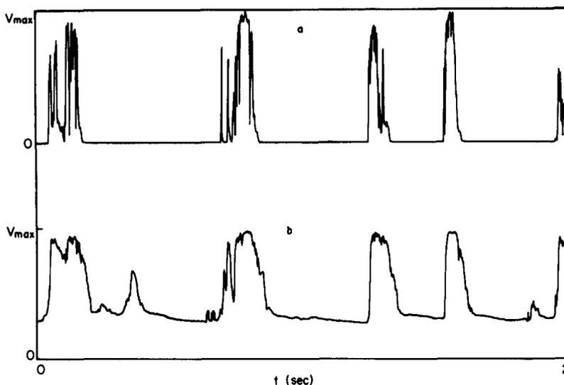
Figure 4. Slug flow,  $u_{Gs} = 4.8$  m/sec,  $u_{Ls} = 1.2$  m/sec, horizontal.
