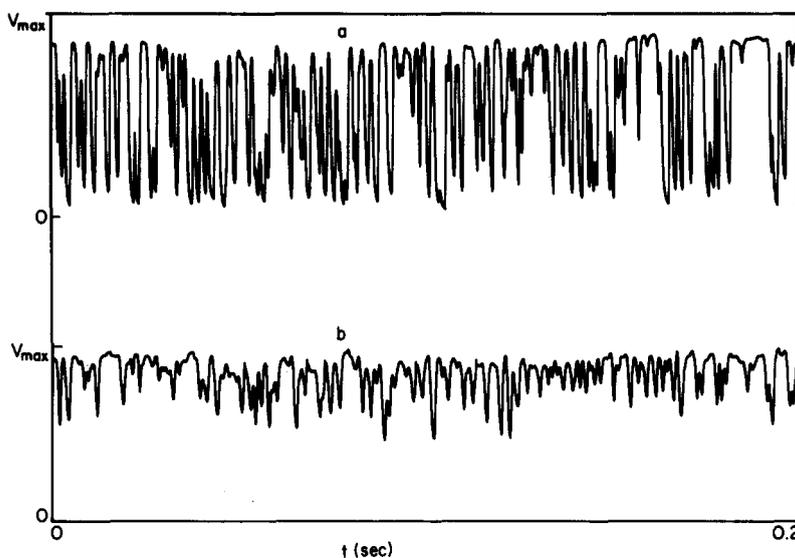
Figure 5. Dispersed bubble flow,  $u_{Gs} = 0.19$  m/sec,  $u_{Ls} = 3$  m/sec, horizontal.
