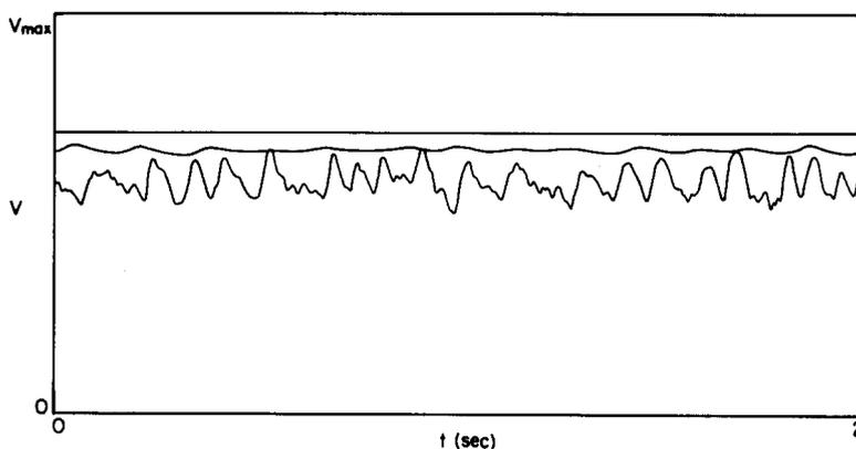
Figure 9. Stratified flow,  $u_{Gs} = 1.2, 3.0$  and  $4.8$  m/sec,  $u_{Ls} = 0.048$  m/sec, horizontal.
