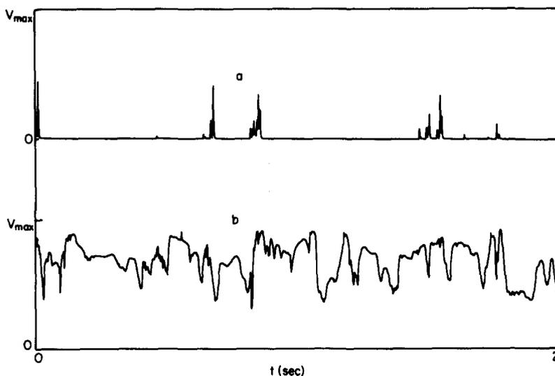
Figure 12. Churn flow,  $u_{Gs} = 7.6$  m/sec,  $u_{Ls} = 0.03$  m/sec, vertical upflow.
