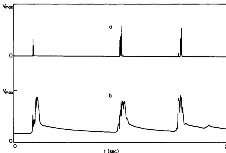
Figure 8. Wavy annular flow,  $u_{Gs} = 4.8$  m/sec,  $u_{Ls} = 0.3$  m/sec, horizontal.
